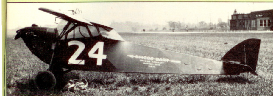
A production model Dart was flown in the 1926 Ford Reliability Tour. The aircraft was powered by a two-cylinder opposed engine rather than the earlier four-cylinder engine.
