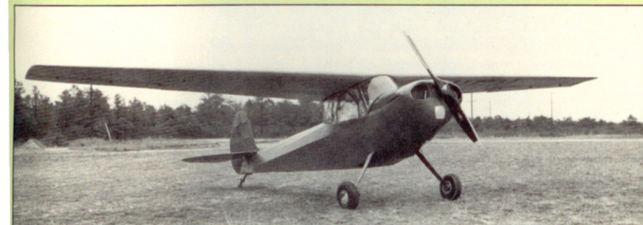
Jack McRae's Super Dart was a modern-day, home-built version of the classic DJ-1. The aircraft had a maximum speed of 125 mph and used a 55-hp Lycoming O-145 powerplant.
