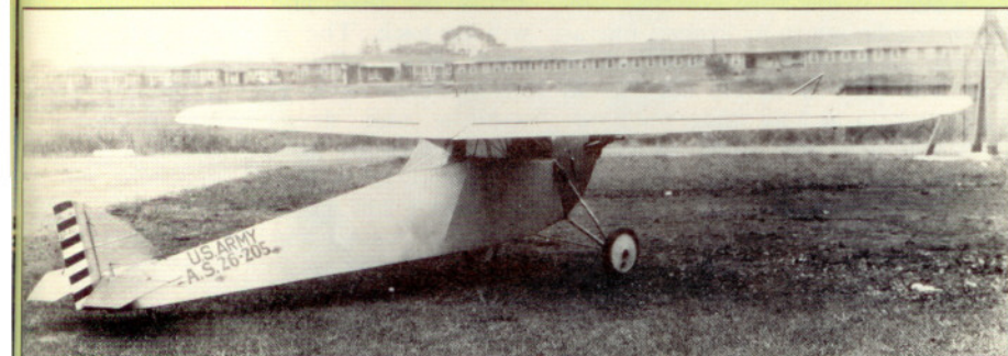
The U.S. Army Air Corps tested a Dart that used flaps and featured droopable ailerons. Leading-edge slots also were incorporated into the aircraft design prior to Army tests.
