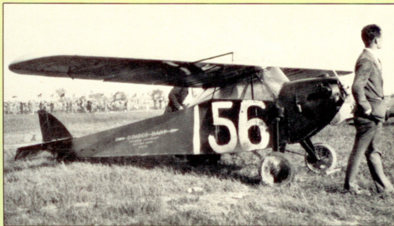
The production Dart (above), flown from Dayton to Philadelphia to participate in the National Air Races in 1926, had a ground-adjustable metal propeller.
